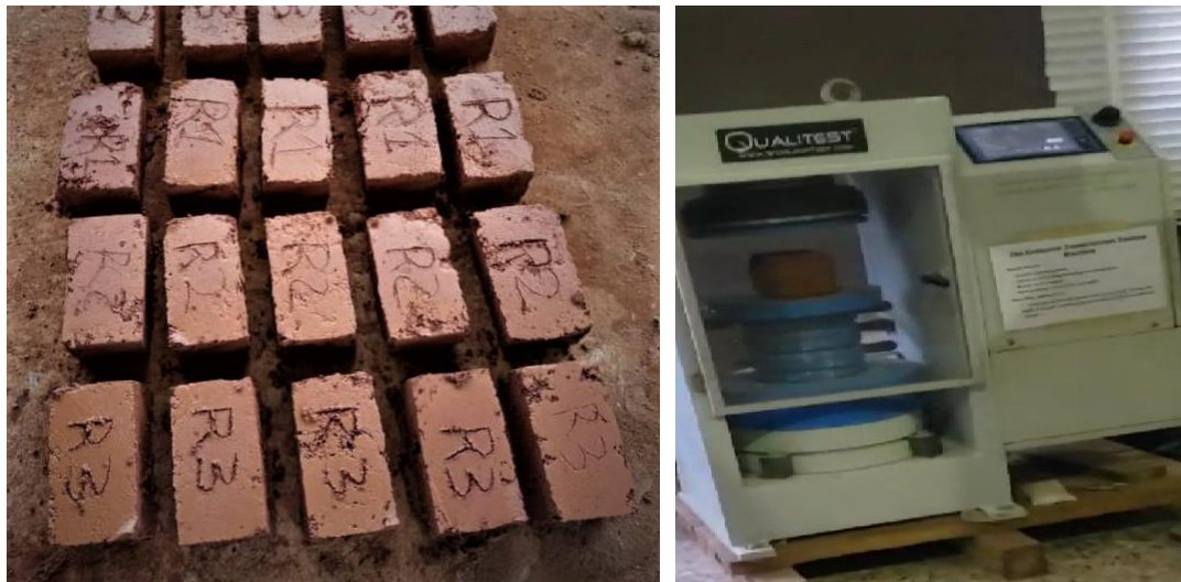
Fig. 2. (a.) freshly moulded block specimen (b.) compressive strength test setup
